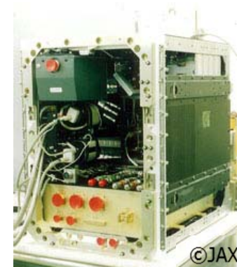
Fluid Physics Experiment Facility
