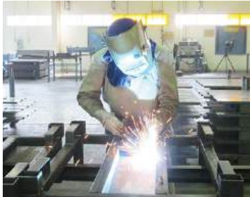
Manufacturing of large pallets for machinery transportation
