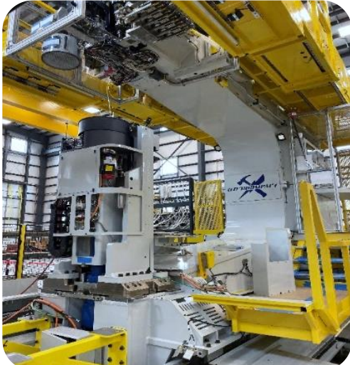
Fuselage Panels (C-Frame Machine)
