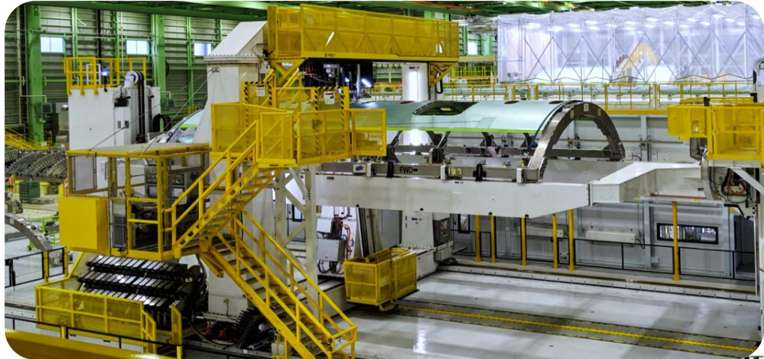
Fuselage Panels (D-Frame Machine)
