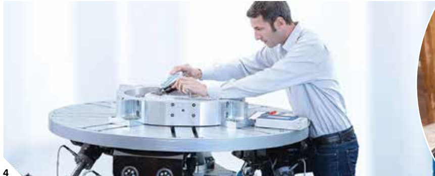
4 // Automatic calibration on hydraulic hexapod at Kistler
