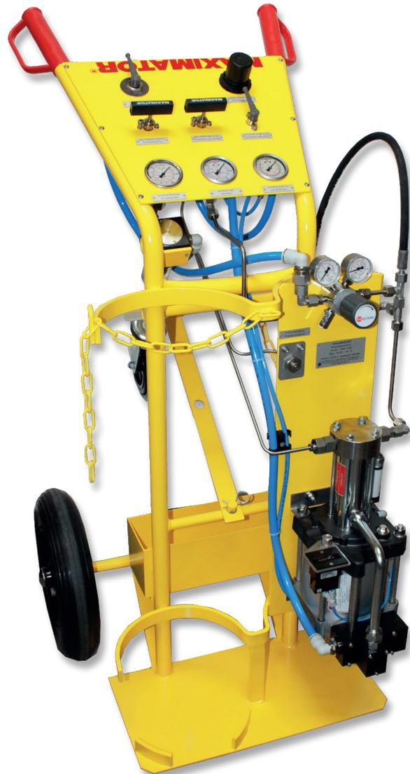
Mobile gas booster cylinder trolley for N<sub>2</sub>-charging applications
