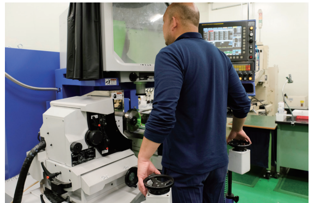
Machining by magnifying 20x or 50x with a projector. The company pursues complex and detailed machining.
