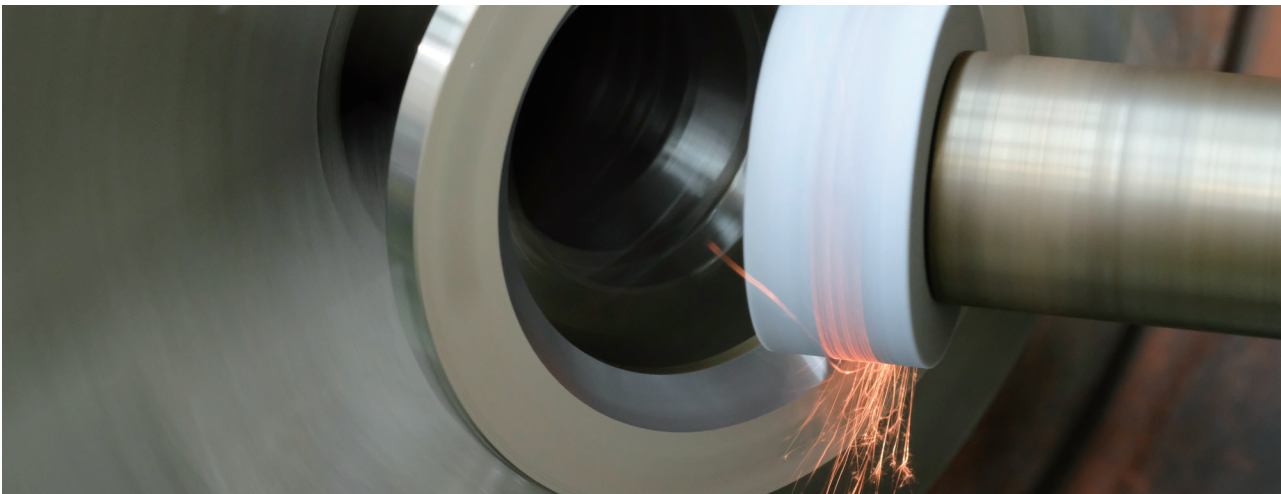
Large diameter \phi 70 70° taper machining. The company has experience machining large objects of more than \phi 200 .
