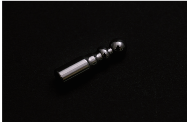
Grinding a sphere (SR, S \phi ) and arc (R)
