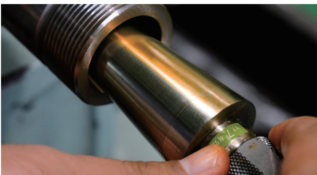
Taper confirmation by fitting. The company aims for more than a 90% match.
