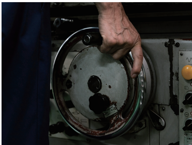
A technician grinds while fine tuning using a handle.
