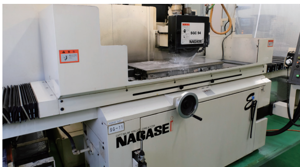
Photograph of surface grinding We handle dovetail groove processing.
