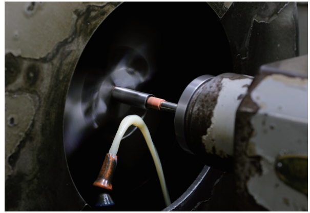
Inner diameter machining from \phi 1 to small diameters is possible.
