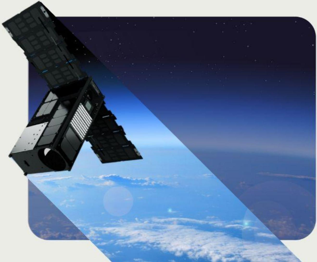
Wyvern hyperspectral sensors on the Dragonette satellites will capture data across many narrow spectral bands, allowing for the specific identification of unique chemical and physical properties of the Earth's surface.
