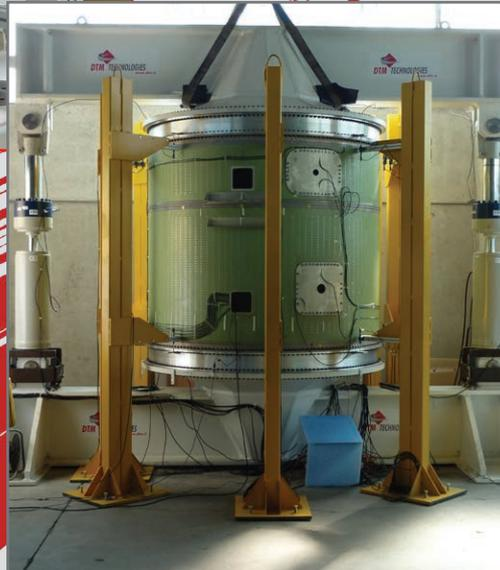
DTM designs and develops custom test jigs to qualify flight structures like the Tank Support Structure of Sentinel 1 (Thales Alenia Space Rome), Vega Interstage 2/3 and composite outer structures of sub-orbital launchers (Swedish Space Corporation)
