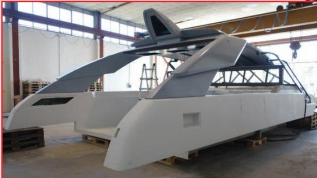
CTop for the Riva76 during assembly at DTM, with a close-up of the large carbon fibre rollbar, designed to overcome a very high first natural frequency value.
