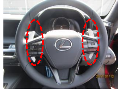
Paddle shift (prototype) Material: AZ91D.
